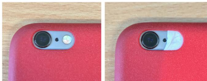
**Figure 1** iPhone 6 back camera before (left) and after (right) flash was covered with some paper tissue. The thickness of the paper tissue used will determine the number of layers of paper to be used. The target was to have a faint flashlight that would be tolerated by a non-sedated horse.
